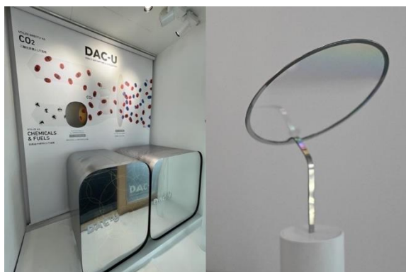
Fig. 1. A prototype of Kyushu University’s Direct Air Capture and Utilization (DAC-U ® ) device (left) and its ultra-thin nanomembrane (right).
